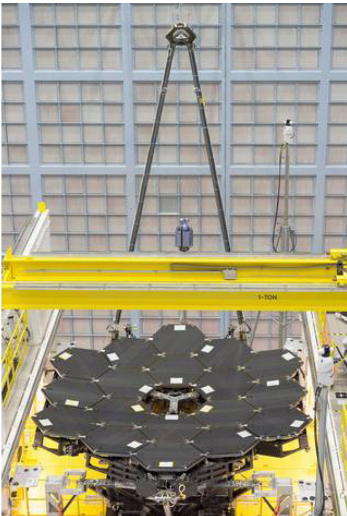
JWST’s 18 mirrors are fully installed on the telescope structure at GSFC. Image credit: NASA / Chris Gunn
