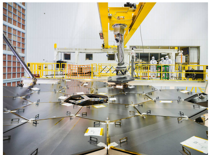
Installation of the last of the telescope’s 18 flight mirrors onto the telescope structure. Each of the mirrors has a protective cover. Image credit: NASA/Chris Gunn
