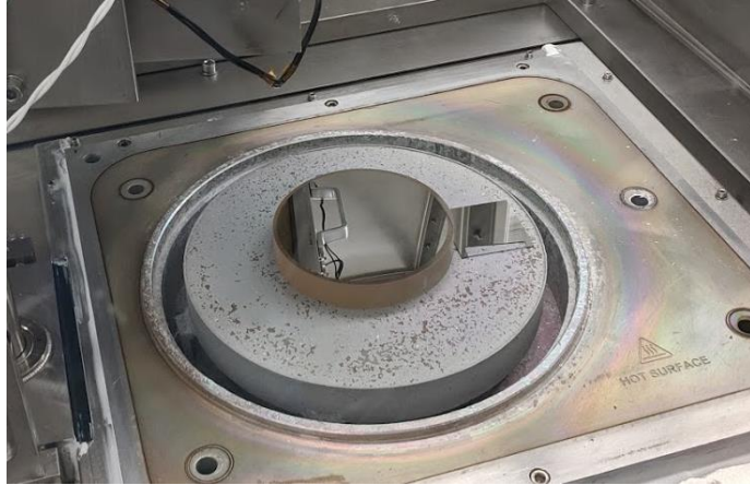
100 mm convex SISTINE secondary overcoated at JPL
