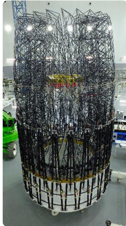
QM of Primary Mirror backplane assembly, 2021
