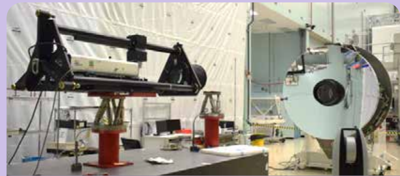
Primary Mirror horizontal optical test
