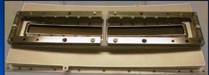
HST-COS far-ultraviolet detector showing the two abutting microchannel plate detector segments (each 85 x 10 mm) curved to the focal plane of the spectrograph.
