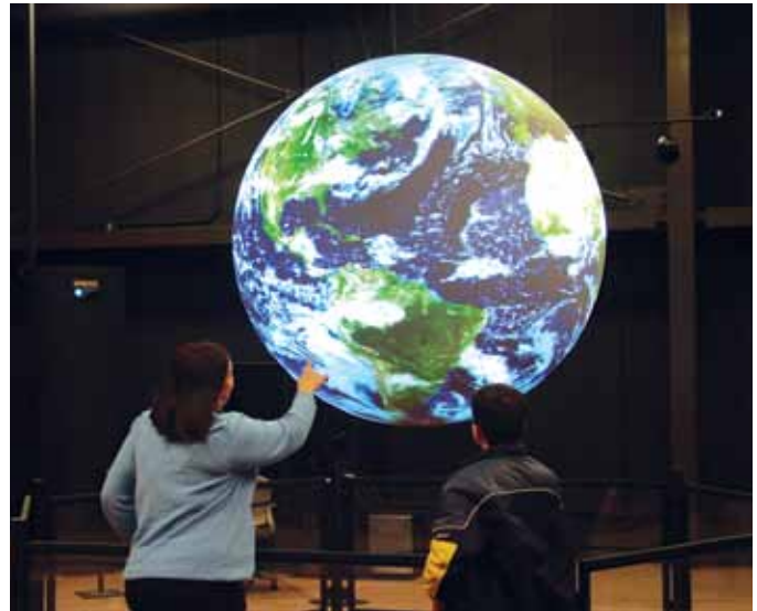
Science On a Sphere® is a room-sized, global display system that uses computers and video projectors to display planetary data onto a six foot diameter sphere, analogous to a giant animated globe. Image credit: NASA
