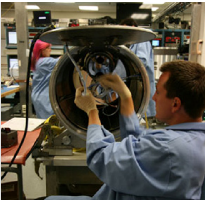
Dr. Brian Hicks, then-UMass Lowell postdoc (now at Goddard Space Flight Center), works on installing shutter door cables during integration at the Wallops Flight Facility.
