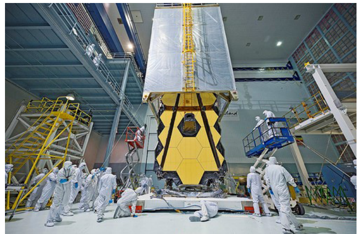
A clean tent is carefully lowered into place around the folded JWST telescope structure, December 2016, in preparation for acoustic and vibration testing. Image credit: NASA/Goddard/Chris Gunn
