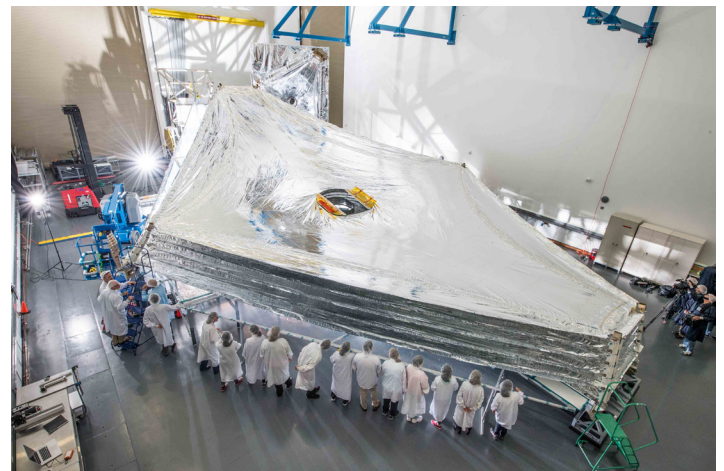
Deployment of a full-sized test sunshield. Image credit: Northrup Grumman
