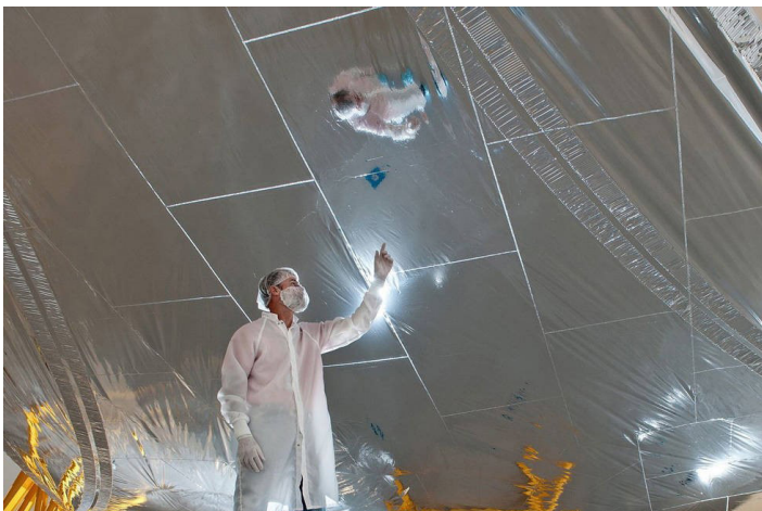
An engineer in a cleanroom looks at one of the sunshield layers that shows a grid pattern of "rip-stops." Credits: Nexvolve
