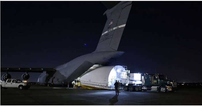
The James Webb Space Telescope has moved to NASA's Johnson Space Center in Houston, TX in May 2017 for the next big test - the cryogenic vacuum test in the Apollo-made-famous Chamber A. The telescope was placed into a climate-controlled container called STARS and loaded into a C-5 cargo airplane. It was unpacked at NASA Johnson. Credits: NASA/ Sophia Roberts
