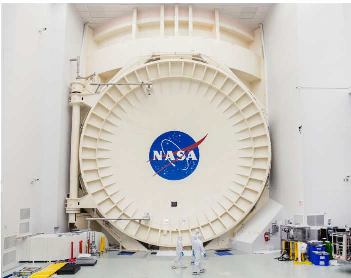
The vault-like 40 foot diameter, 40 ton entry door to Chamber A towers over engineers at Johnson Space Center in Houston. It was sealed shut on 11/07/2017, to start the 93 day final thermal vacuum test for the Webb Optical Telescope + ISIM (OTIS). Image credit: NASA/Chris Gunn
