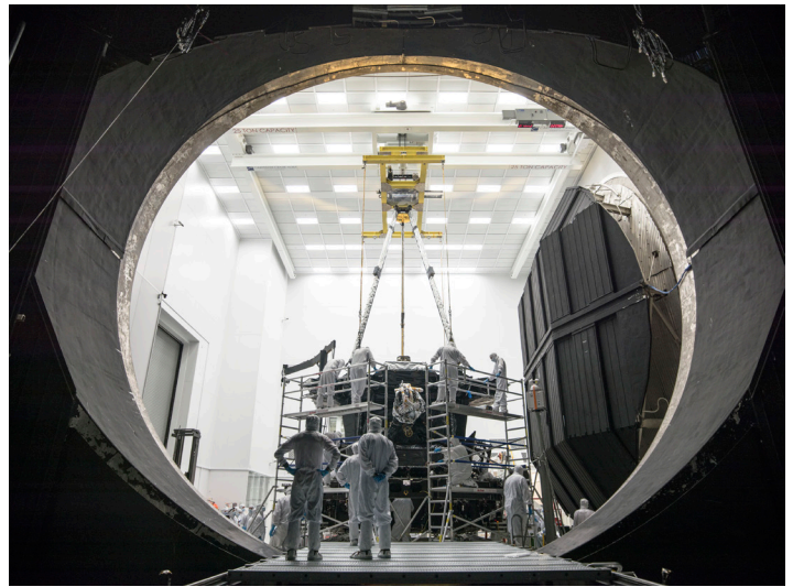
This image, taken from inside the NASA Johnson Space Center Chamber A, captures the James Webb Space Telescope being lifted onto its test stand before sliding it into the chamber. Credits: NASA/Chris Gunn
