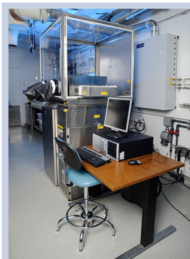
Fig 11. ALD coating system at JPL; gas feed-throughs and process controls enable AlF 3 and MgF 2 coatings development.
