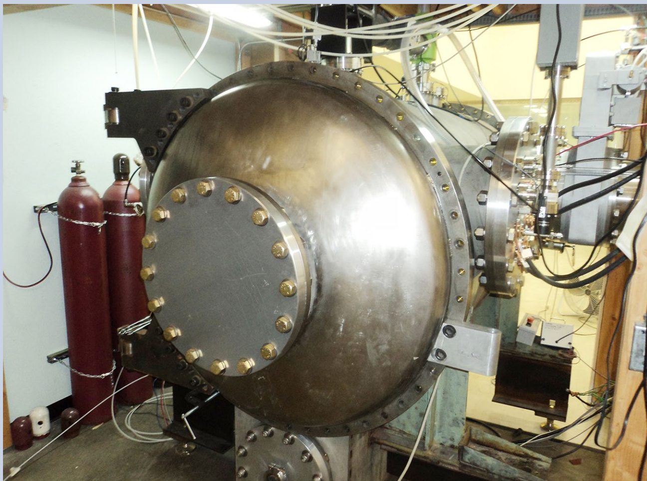
Fig. 1. A 1.2 m coating chamber fitted with process controllers, thickness monitor, and gas analyzer (courtesy: Zecoat Corp).
