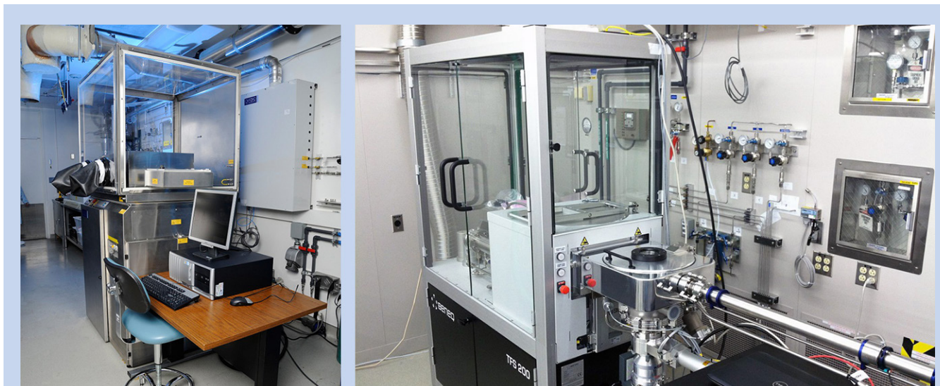
Fig. 6. ALD systems at JPL. Left: Oxford OpAl showerhead-style ALD reactor with gas feedthroughs and process controls enabling \text{AlF}_3 and \text{MgF}_2 coatings development. Right: Beneq ALD deposition system.
