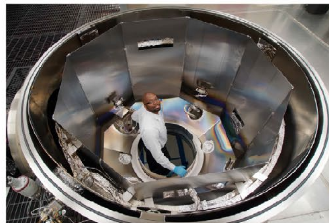
Inside 2-meter coating chamber after installation of thermal shroud and halogen-quartz heater lamps.
