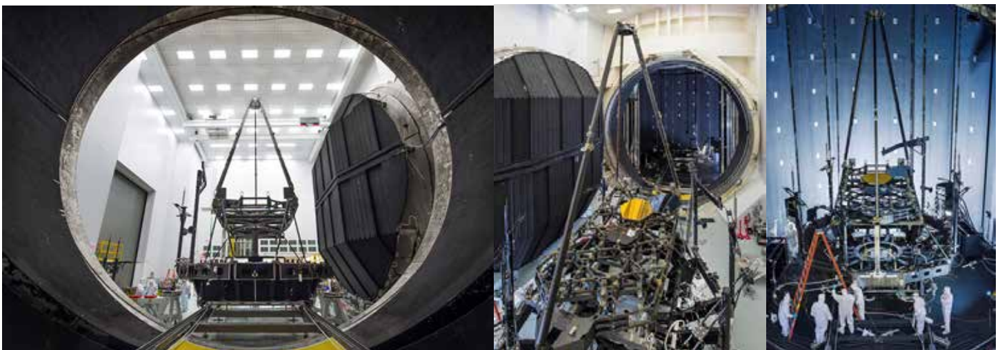
(Left and center) The JWST Pathfinder prepares for a fit-check in Johnson Space Flight Center's Chamber A, in April 2015. It cleared the chamber door by 8 inches. Image credit: Chris Gunn, (Right) The JWST Pathfinder backplane test model is prepared for its cryogenic test in Chamber A at Johnson Space Center in Houston. This was the first time two mirror segments were aligned together, as part of a larger optical surface. The test was successfully completed in May.
