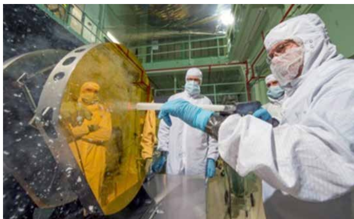
Test of the cleaning on the SBMD mirror on January 22, 2015. Bill Ryan of Harris performs the procedure with Jim Collins and Matt Magsamen looking on.
