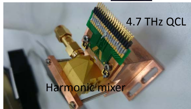
Array of DFB lasers at ~4.7 THz. The harmonic mixer is used to phase lock the QCL LO.
