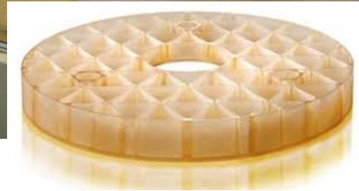
1.2m Schott mirror ready for polish & mounting structure
